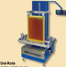
provides a reliable, low-cost option for automating screen coating. Front and rear screen coaters can apply emulsion in tandem or independently, allowing operators to coat each side of the screen separately, both sides simultaneously, or just one side. M&R's Job Recall™ allows users to save up to five screen coating jobs for added convenience and quick changeover.
